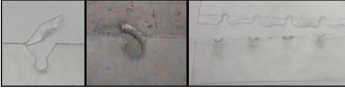
Figure 4. Laminate edge failure mechanisms.
