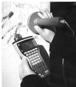
Corrosion activity being evaluated on a bridge wall with the GalvaPulse
