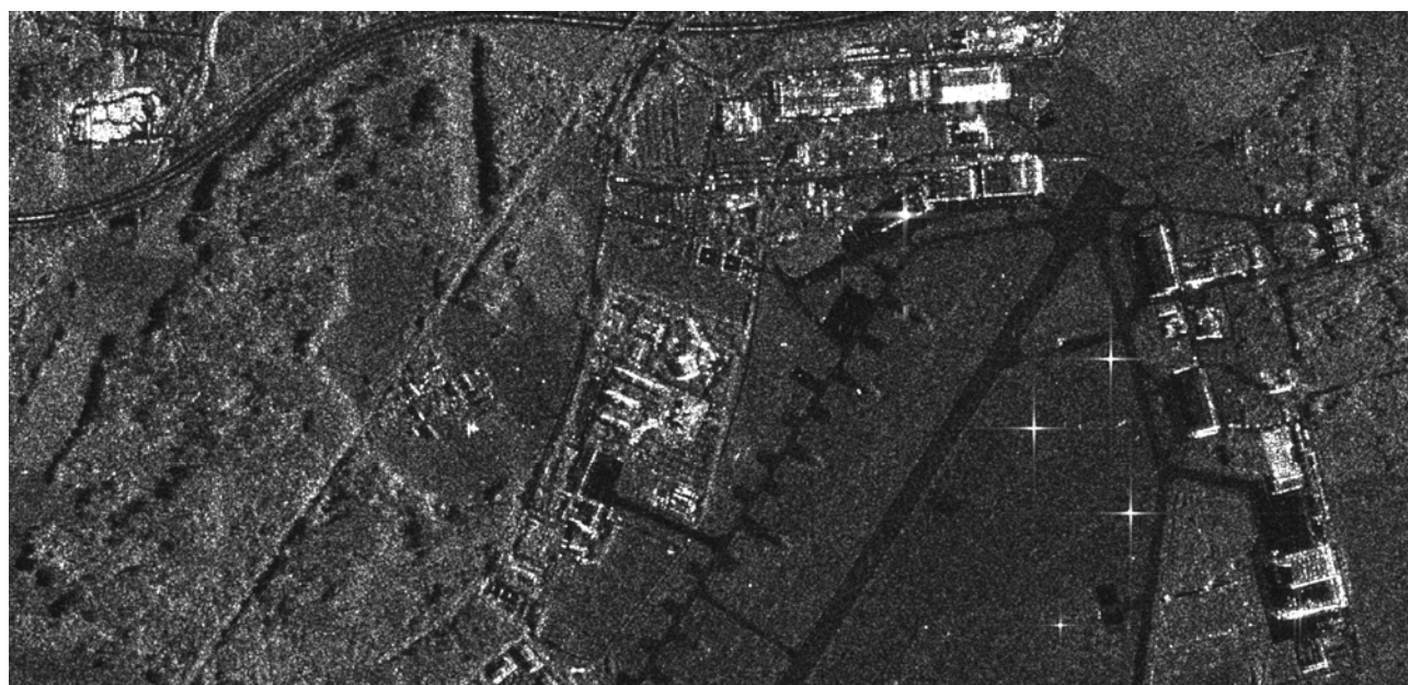
Fig. 3-1: Example for a spatially enhanced stripmap product with 1.2 looks and approx. 3.2 meter resolution of the Oberpfaffenhofen calibration site. The extent is 2.9km x 1.4km (pixel spacing: 1.25m)
