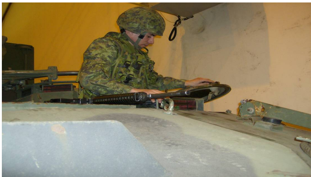
Figure 52: Bison Driver Getting into the Drivers Station
