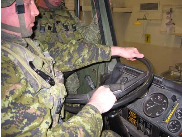
Figure 21: Tactical Vest Interference with Steering Wheel
