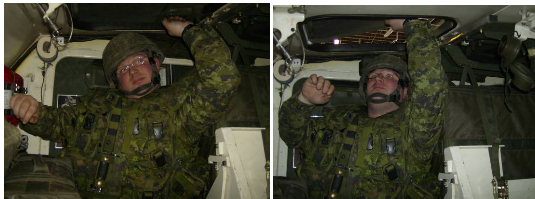
Figure 80: Coyote Operator Egress Through Family Hatch
