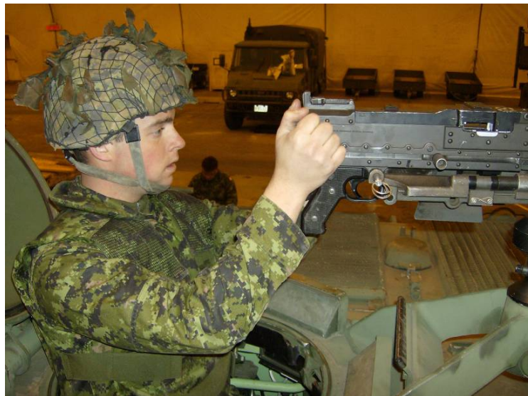
Figure 39: TLAV CC Demonstrating Arm Position When Using Spade Grips
