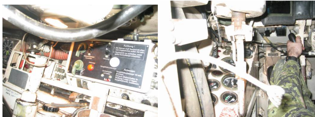
Figure 62: Leopard Driver Control Buttons, a) on the right side, b) on the left side
