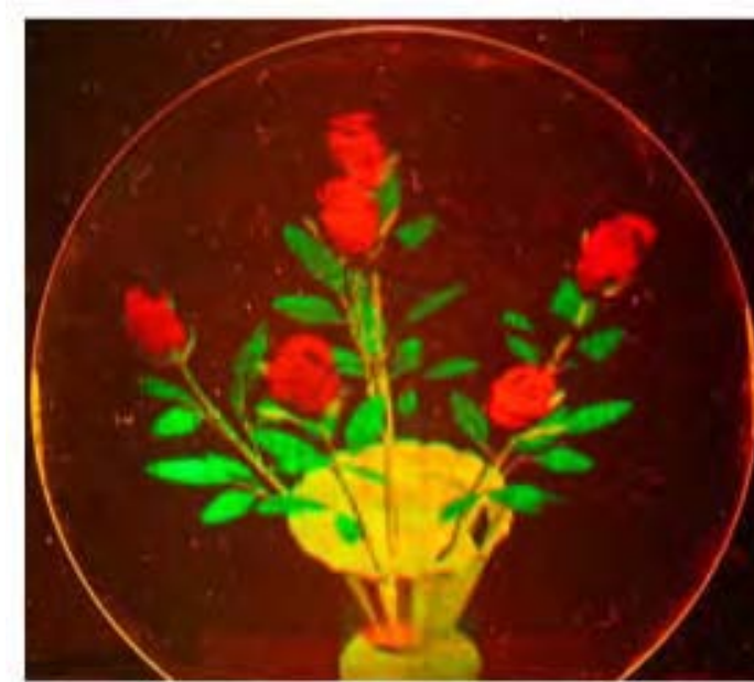
Figure 14. Example of two color holograms. Compared to our previous technique, we see that the color hologram efficiency is higher, colors crispier and color mixing smoother. One can see how the vase is uniformly gold due to the combined diffraction of the green and red holograms.
