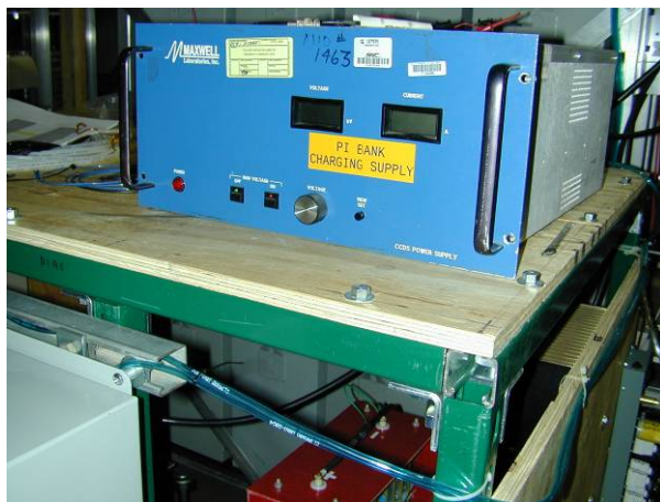
Figure 71. (a) PI bank CCS power supply; (b) interface box
