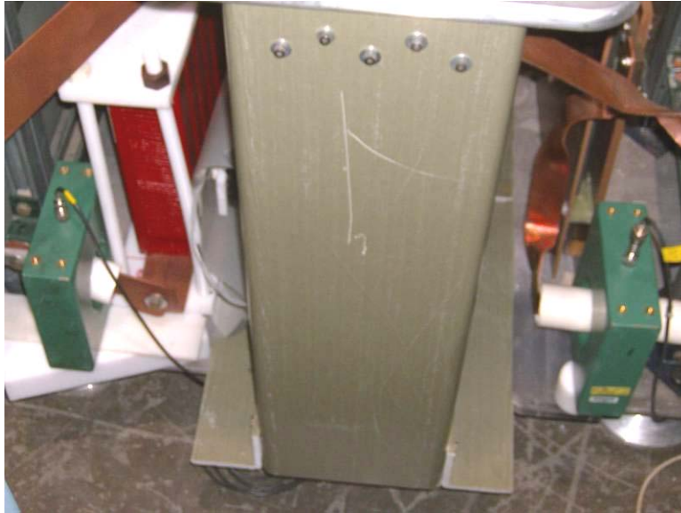
Figure 40. Pearson Model 1423s installed on each bank module
