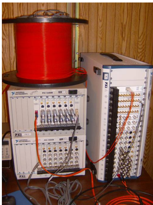
Figure 63. 18-slot PXI crate (right) and two 8-slot crates (left)
