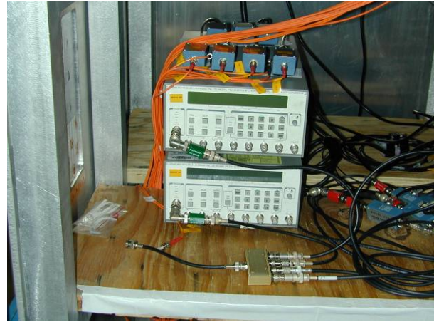
Figure 64. (a) New cable tray and fiber-optic feedthroughs; (b) DG-535s
