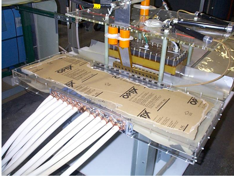
Figure 6. PI bank SF 6 enclosure being test-fitted
