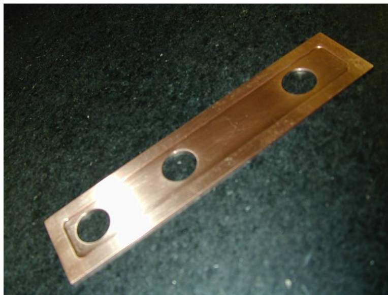
Figure 104. Copper gasket, designed for improved current-joint contact
