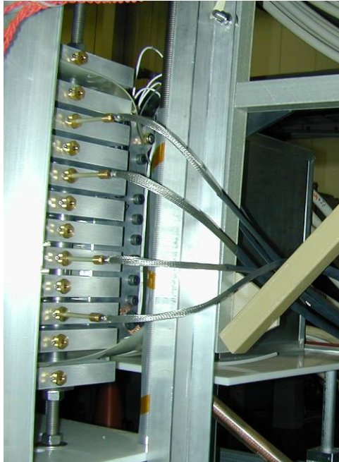
Figure 53. Four B-dot probes in Theta coil, segments B, D, G, and I
