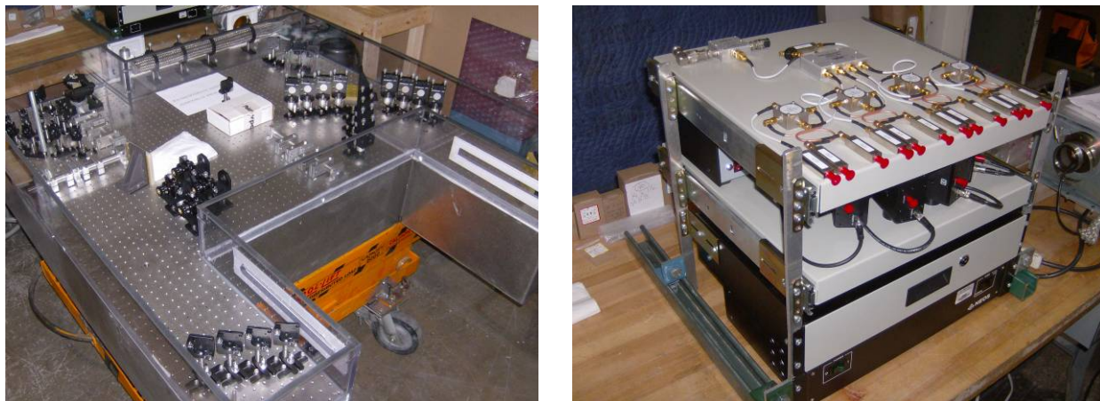
Figure 17. (a) Mounting of opto-mechanical components on optics table; (b) interferometer detectors and RF components
