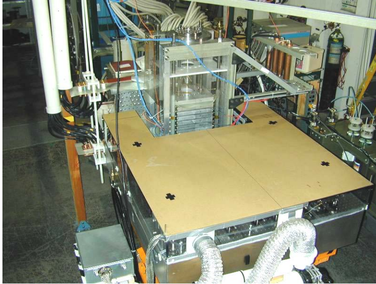
Figure 54. Four-chord interferometer in place around vacuum and field-coil stand Figure 55 shows the interferometer detectors and circuits at the bottom of the remote data acquisition box.
