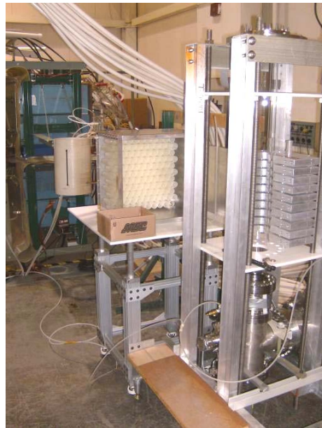
Figure 44. Vertical stand and cable header support table
