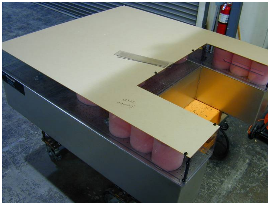
Figure 16. Four-chord interferometer optics table and its dust cover
