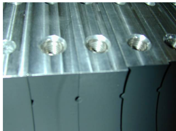
Figure 107. (a) Modified Cusp and Theta coil segments; (b) close-up view of tapped holes added to several coil-segment halves
