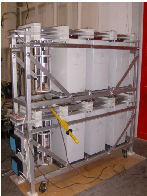
Figure 34. (a) Two 1.5 mF Cusp bank modules stacked on top of each other; (b) ignitron trigger units
