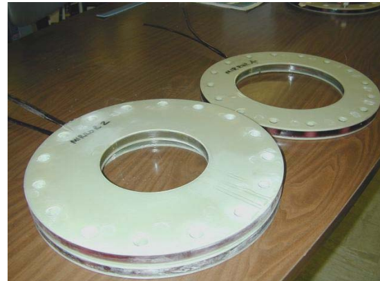
Figure 101. (a) First mirror coil; (b) several coils in G-10 spools
