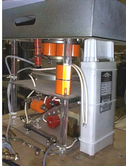
Figure 10. Maxwell 40151-B trigger generator with additional 100 kV, 0.099 \mu\text{F} capacitor
