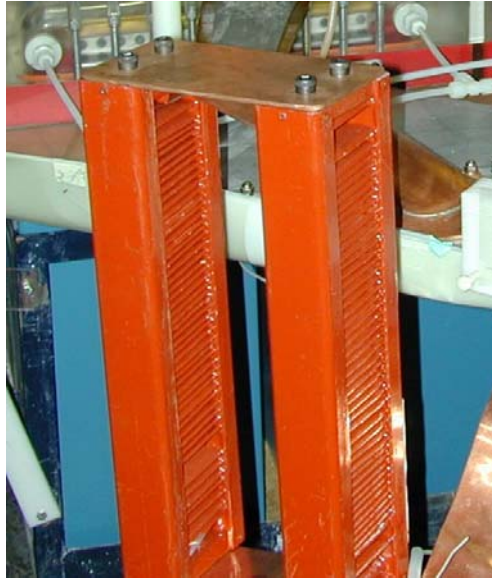
Figure C2. Franklin resistors that are commonly used in-house
