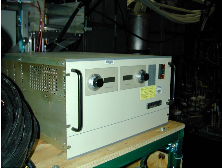
Figure 108. 100 kV, 60 mA, negative polarity Spellman power supply
