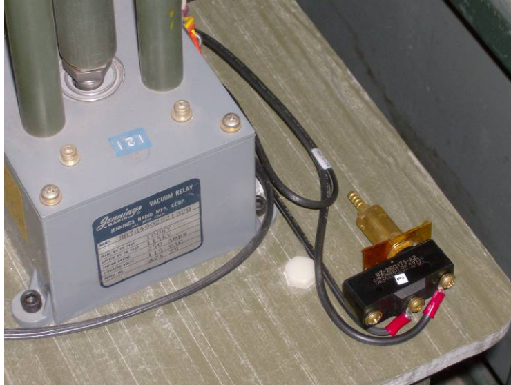
Figure 70. Clippard pneumatically-actuated switches
