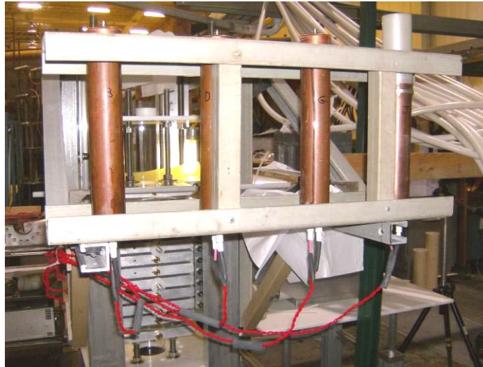
Figure 52. Flux-loop voltage dividers in fiberglass frame
