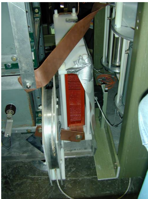
Figure 26. Copper bus straps, damping resistor, and ignitron (upper right) for second Bias bank module
