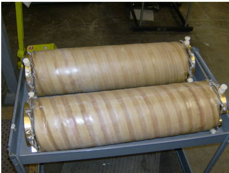
Figure 30. New Bias bank isolation inductors
