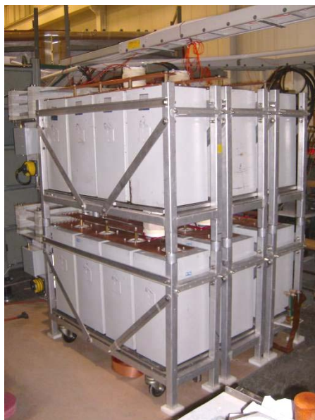
Figure 97. Guide/Mirror bank modules, stacked two-high
