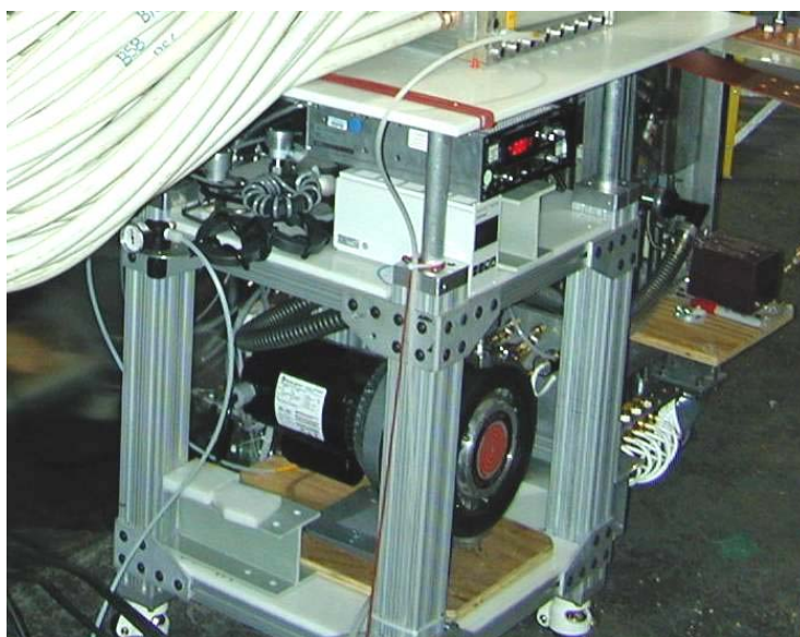
Figure 46. Roughing pump and vacuum-gauge controllers beneath Theta coil cable header A second shelf was placed above the mechanical pump as a place to mount the vacuum gauge controllers and the various valves and components for the deuterium and dry nitrogen systems. (See Section 4.2.4.)
