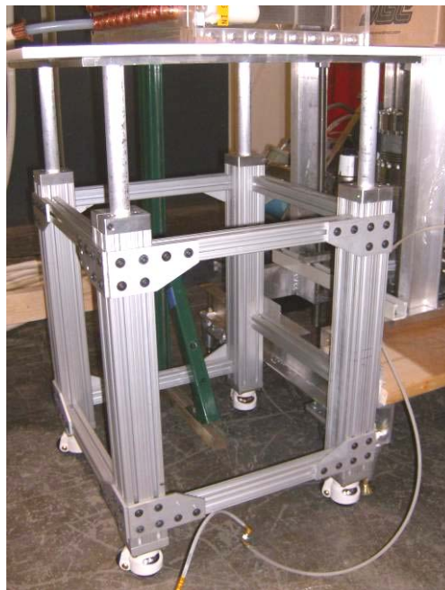
Figure 43. Completed Theta coil cable header support table
