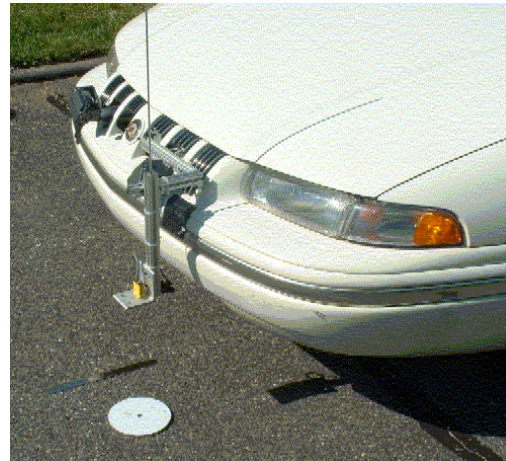
Figure 1 Note the downward looking photo sensor, the retroreflector on the ground and the vertical rod to guide the driver.
