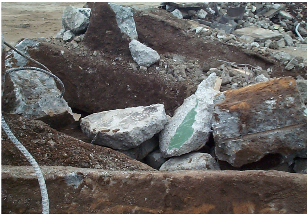
Figure 13. LBP covered concrete in mixed debris pile.
