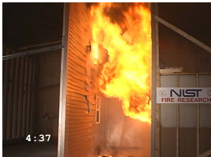
In a NIST lab test, flames from a simulated house with combustibile exterior walls ignite a similar "house" six feet away. The numbers in the corner are the time (in minutes) since the start of the test. (Photo courtesy of National Institute of Standards and Technology)
