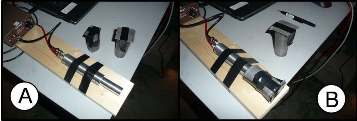
Fig. 53 The LaBr scintillator was mounted to a board which was placed into the pile. This allowed the detector to be replaced in the same location each time it was removed. The detector was placed into the pile without any covering 'A' and with both Lead and Cadmium shields both of which are shown in 'B'.
