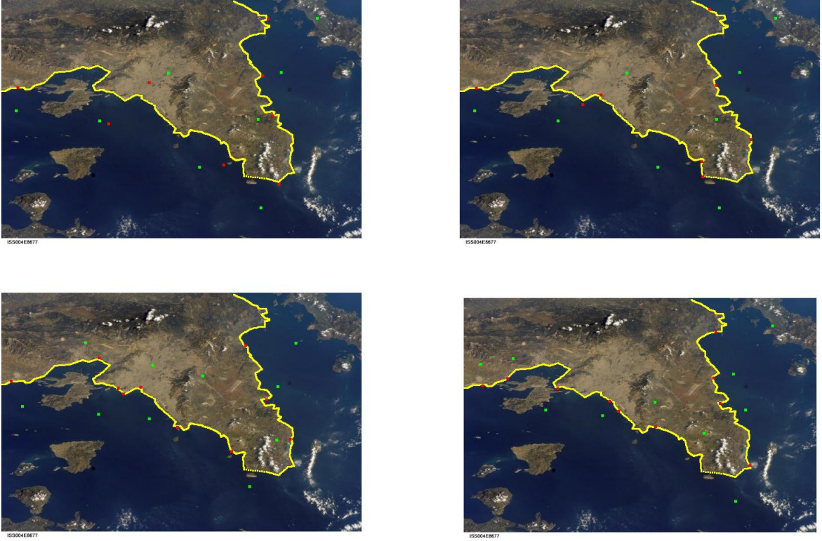
Fig. 3. Examples of placing the sensors in a curve, the yellow line. Results for two different values of \lambda are shown in the first row, with a higher value on the right (note how all the sensors are located on the yellow line). A different distances configuration is shown in the second row, left. In the second row, right, an additional example is shown, where some of the pairwise distances between the sensors are not available ( w_{ij} = 0 in Equation (1)).
