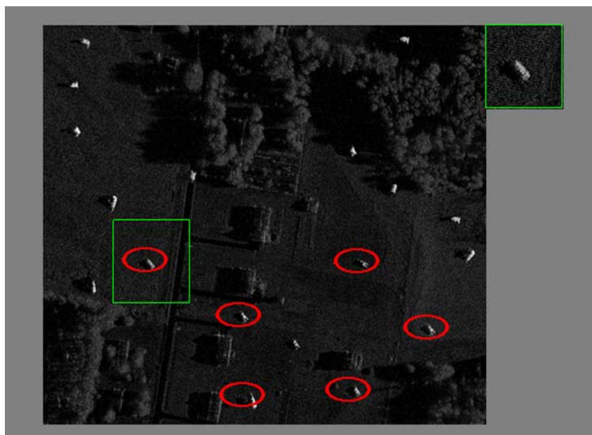
Figure 3. An example of a side window magnifier. The green square at the left is the area that is magnified in the window on the right
