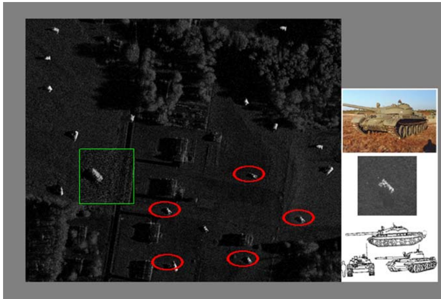
Figure 4. An example of a display with a moving magnifier together with an information window. In addition to the green square on the left where the magnification occurs, on the left we see the information window with information about the enlarged vehicle. This vehicle was designated by the ATR so that a press of the right button displayed information about it
