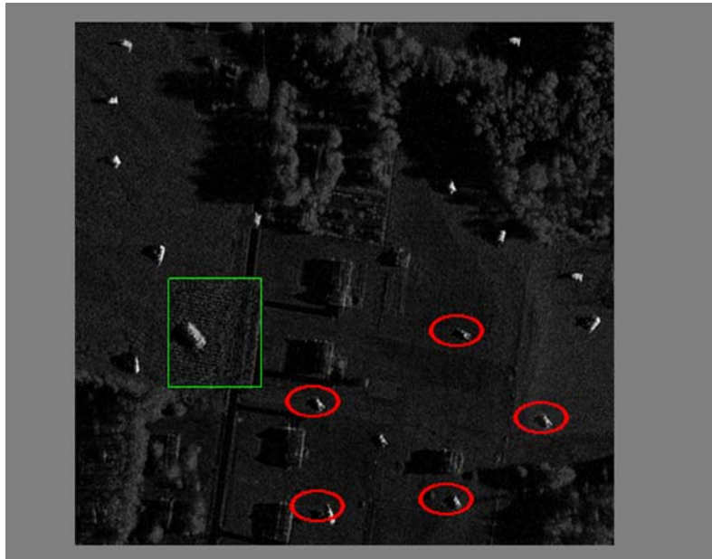
Figure 2. An example of a moving magnifier image. The green square at the left is the magnification, where the vehicle within it is magnified by 2 compared to the other vehicles in the image. The red ellipses are a simulation of the ATR designations
