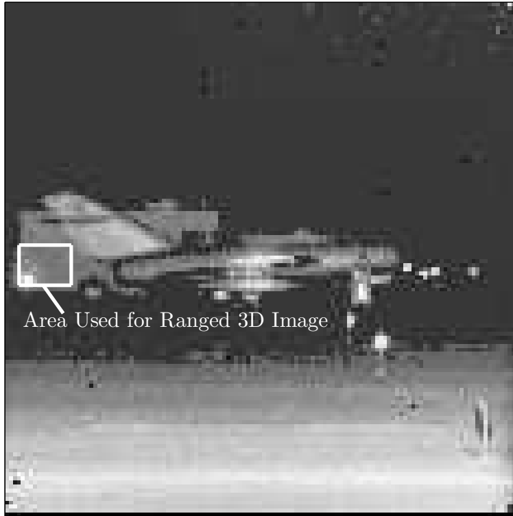
Figure 33: An intensity LADAR image showing the portion of the van used to discuss saturation effects on range estimation
