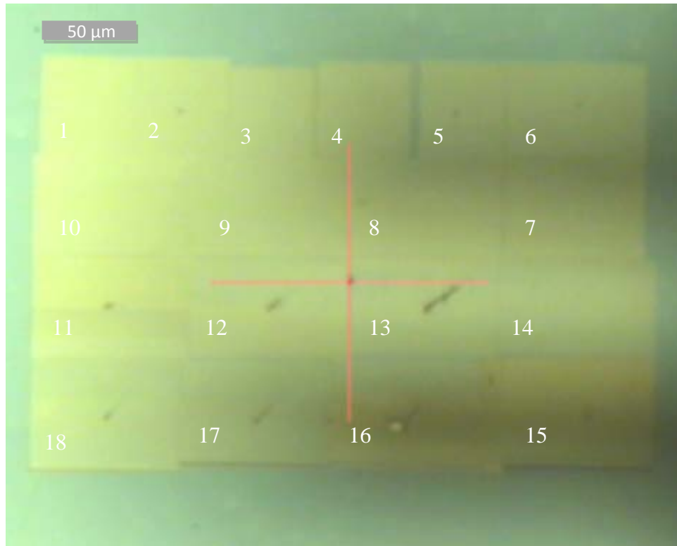
Figure 10: Completed AFM-patterned 2-D thin-film photonic crystal (each pattern is numbered in lower left corner in the order they were produced)
