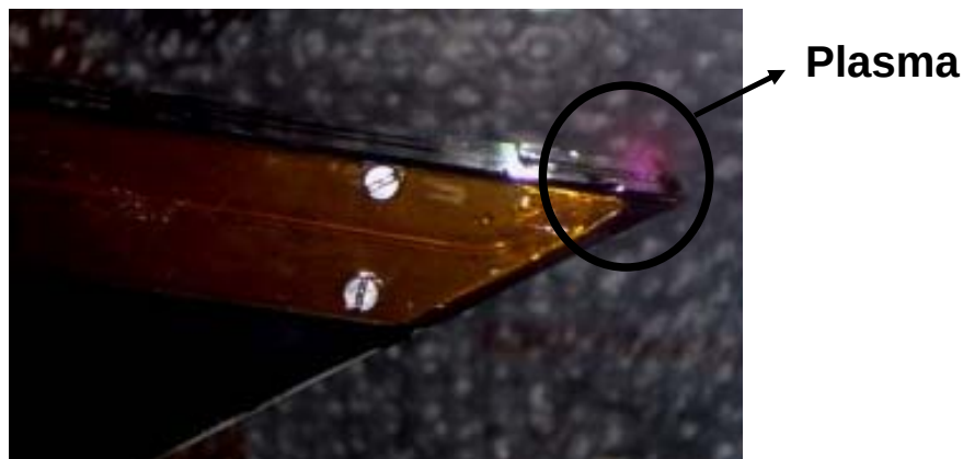
Figure.8: Photograph of the plasma on the model surface near the leading edge
