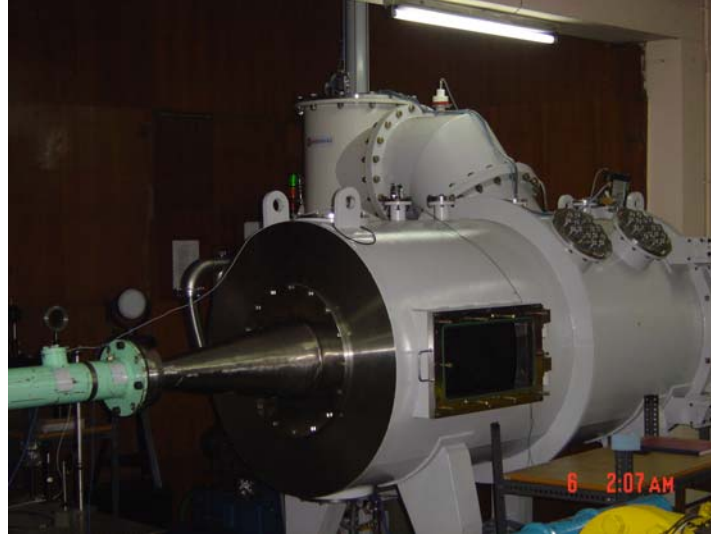
Fig.1: Photograph showing the tunnel portion of the HST5 shock tunnel.
