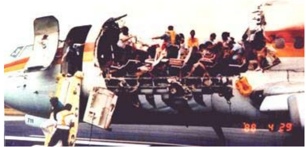
Figure 11 Aloha Airlines Flight 811 multi-site crack damage torn away the top of the aircraft skin
