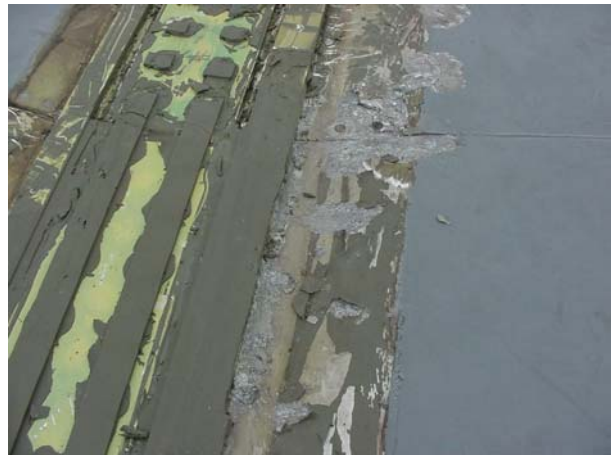
Figure 12 Service damage on aircraft skin
