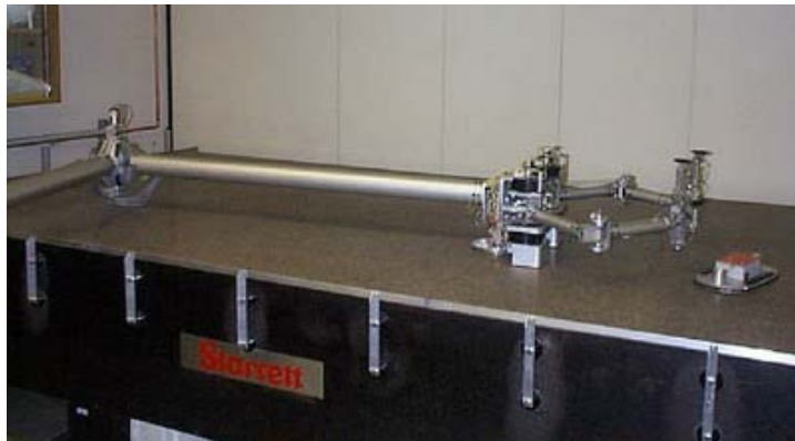
Figure 2.1: Two-Link Manipulator Testbed at Stanford University’s ARL [43]
