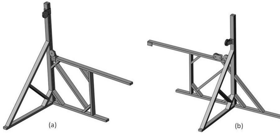
Figure 3.13: Loading Structure - (a) Qualification and (b) Joined-wing.
