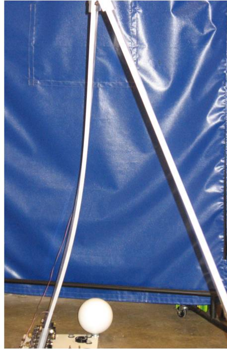
Figure 4.55: Solid Joined-wing - Test Article under a 1,000 lb Load.
