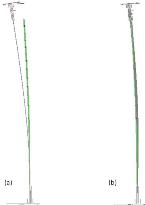
Figure B.7: Solid Qualification - Transverse Bending - 1100 lb Surface Matching - (a) Linear and (b) Non-Linear.
