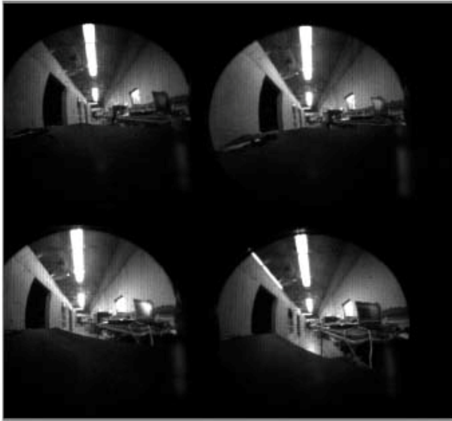
Figure 1. Sample image from Polarization camera system. There are 4 separate fisheye images shown in this one camera image, the result of our quadfricated fiber bundle. Each small fisheye image carries different polarization information. Three of the images have linear polarizers in line with the image optical path. The remaining image contains a circular polarization analyzer. By combining these images, the 4 stokes vectors can be determined.
