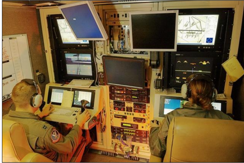
Figure 10. Predator Ground Control Station
