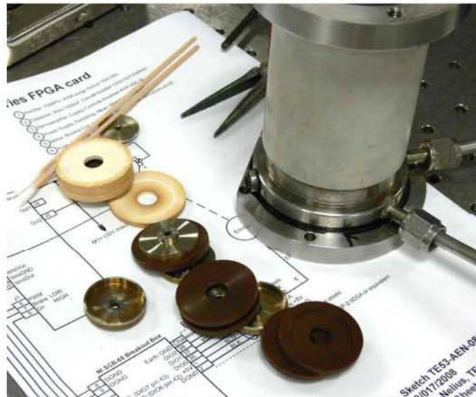
Figure C-3. Pulsed Electron Gun Shown Disassembled.
