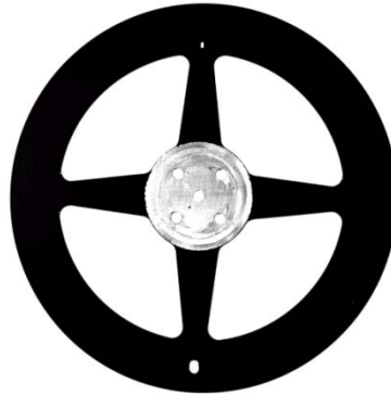
Figure C-12. Photograph of Original Rotating Disk in FARVA Showing 0.125-in.-diam Aperture at Bottom and Smaller Aperture Used for Timing Purposes at Top.
