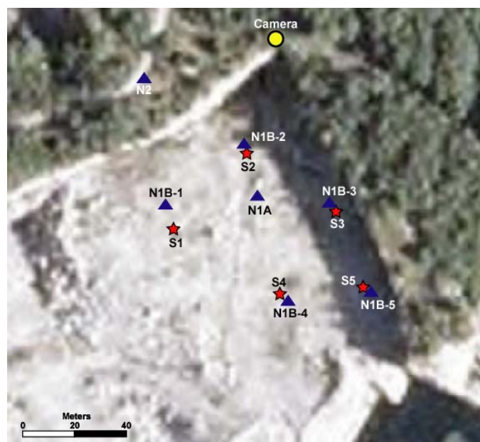
Figure 6. Test site station N1 (blue triangles) and shots (red stars). N1 consisted of two Endevco accelerometers. N1A remained stationary for all 5 shots, while N1B moved to be less than 5 m from each shot. Station N2 and the camera are also shown on a hill overlooking the test site. (Google Earth Background)
