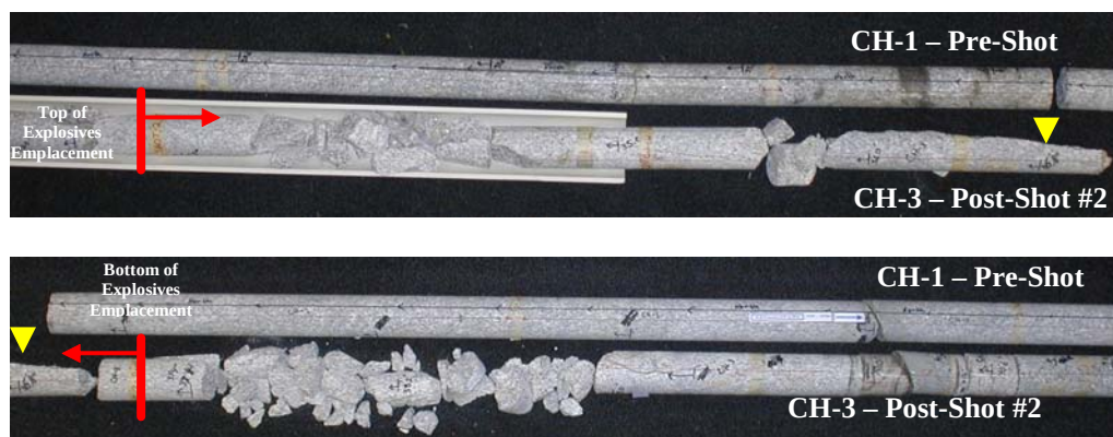
Figure 99. Comparison between cores recovered from the pre-shot and post-shot coreholes adjacent to Shot 2. The explosives emplacement interval was from 33.14 ft to 37.08 ft (10.1 m to 11.3 m).
