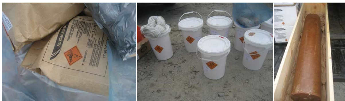
Figure 74. Photo of the explosives used in the NEDE. (Left) Packages of “Polvara Negra” or black powder. (Middle) Containers of pre-mixed Heavy ANFO (50:50 ANFO:Emulsion). (Right) A cast charge of Composition B.
