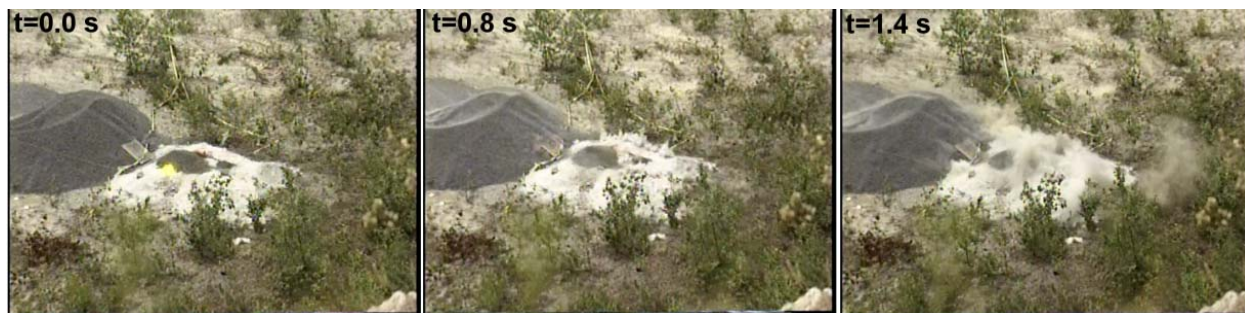
Figure 26. Digitized still images of the Shot 2 detonation. Three fractures develop in the white granite flour at 0.8 s and a larger opening releases a plume of gases to the right of the flour at 1.4 s.
