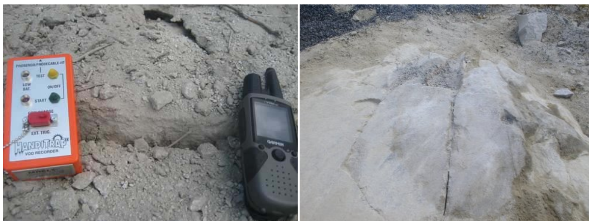
Figure 83. Surficial cracks after the Shot 1 (black powder; left) and Shot 2 (ANFO; right) explosions. The cracks shown at left showed permanent displacement of a few centimeters or more.
