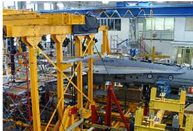
Figure 12: Full-scale fatigue test of CF-18 aircraft [6]
