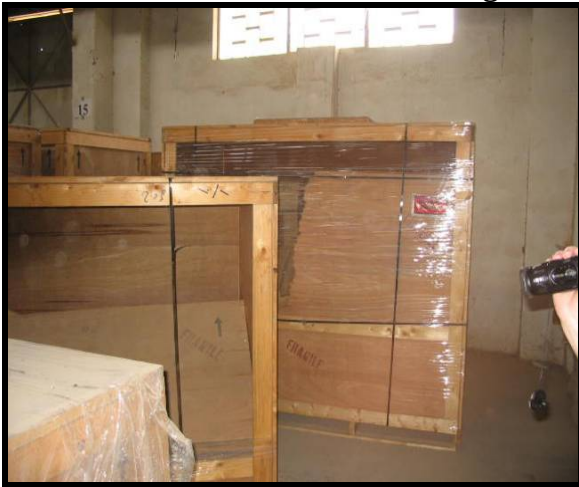
Photo 6. Two crates with Side Panels Missing/Busted
