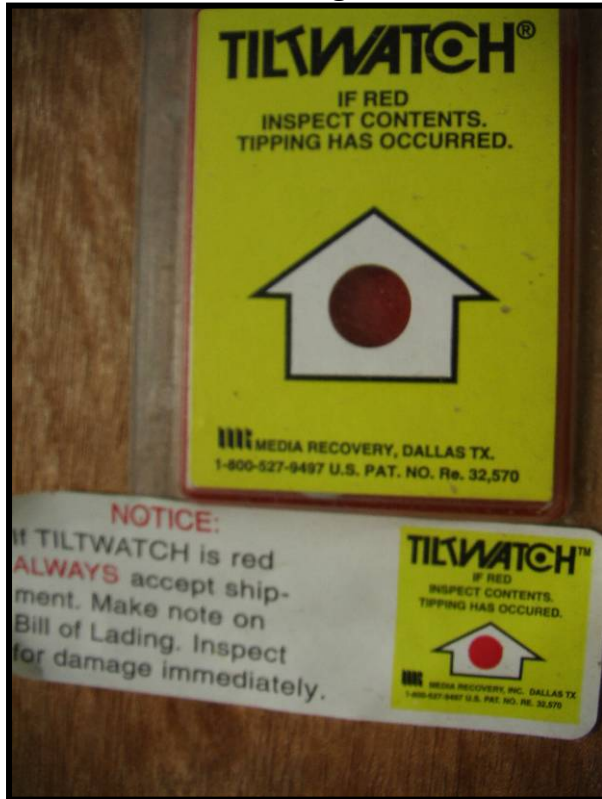
Photo 9. Tiltwatch Meter Showing “Red”
