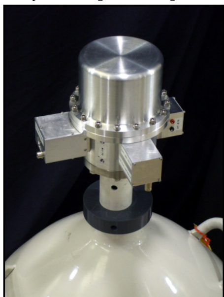
Figure 3. The MJX cryostat holds, cools, and instruments p-type point contact detectors like MJ70.
