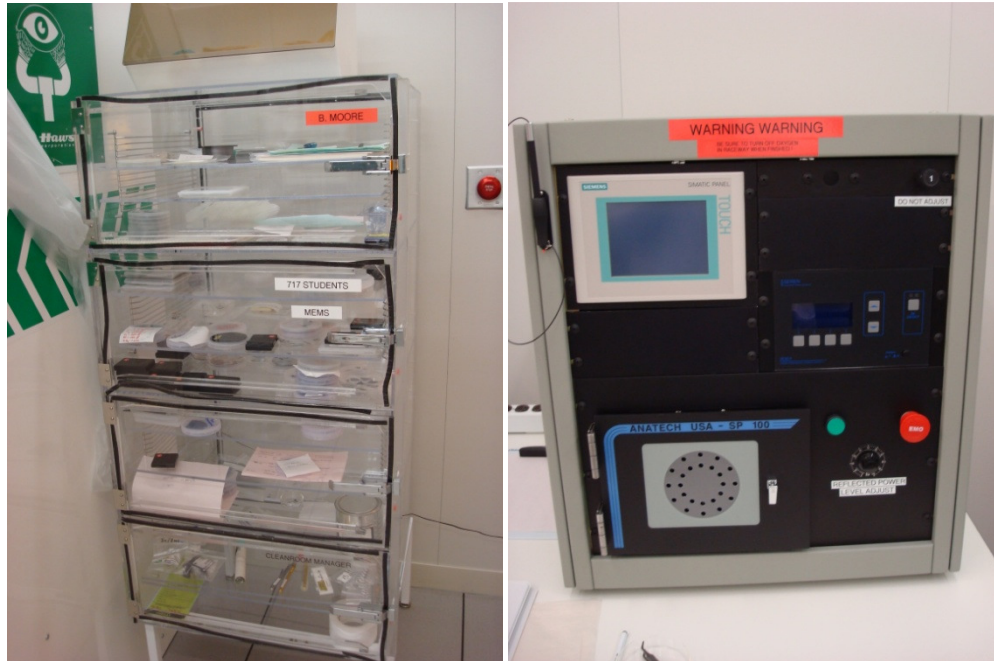
(a) (b) Figure 3.22: Cleanroom dry box (a) and Anatech plasma cleaner (b).
