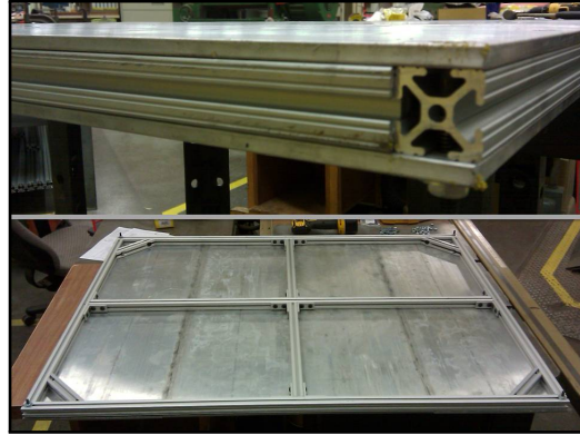
(b) Breadboard with edge close up and internal view
