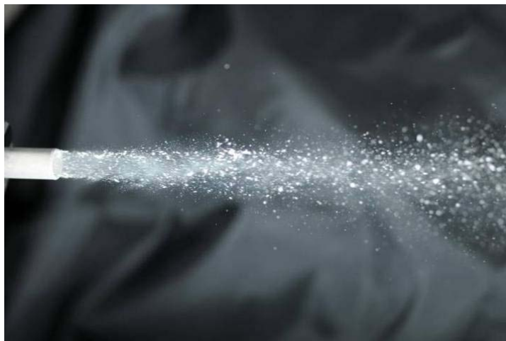
Figure 4.3: Characteristic profile of particles exiting a simple shroud tube.
