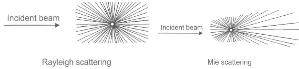
Figure 2.2: Rayleigh and Mie scattering characteristics. [12]
