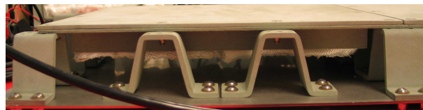
Figure 6: Side View of Physical TPS
