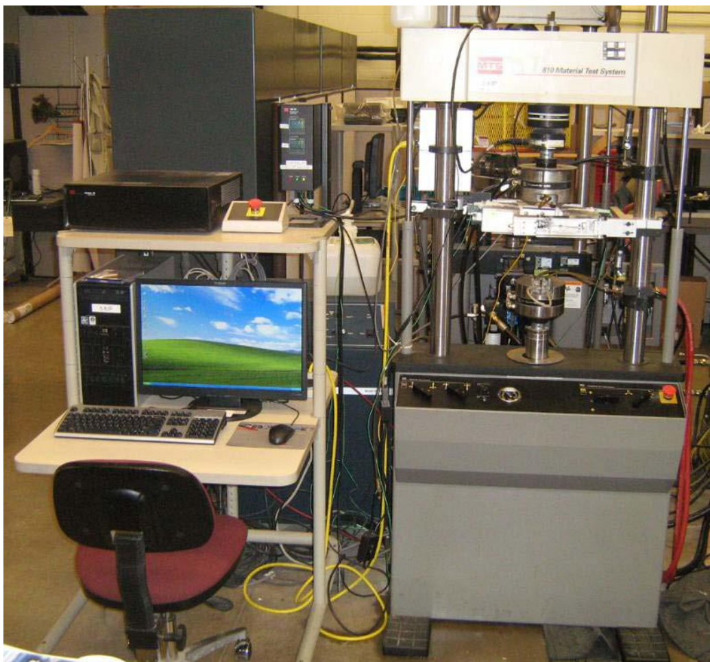
Figure 13: MTS 5 Kip machine.
