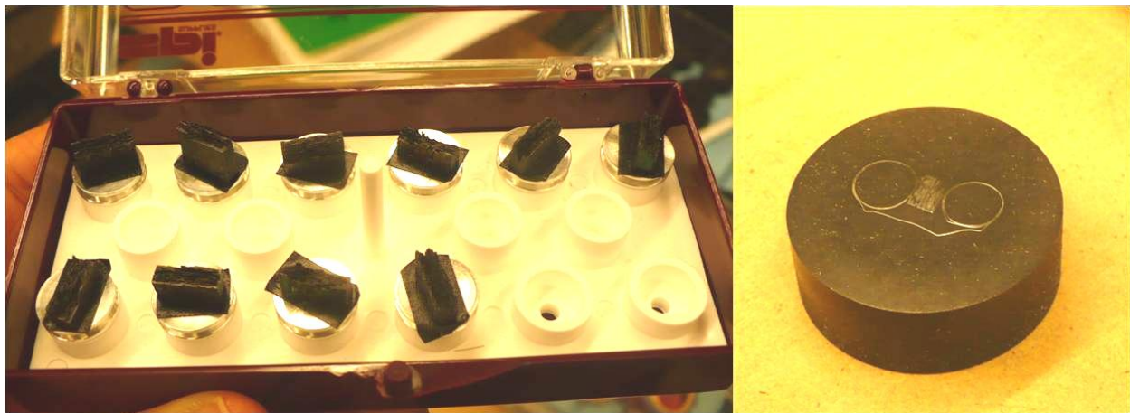
Figure 19: Hi-Nicalon/PyC/SiC specimens prepared for SEM observation.
