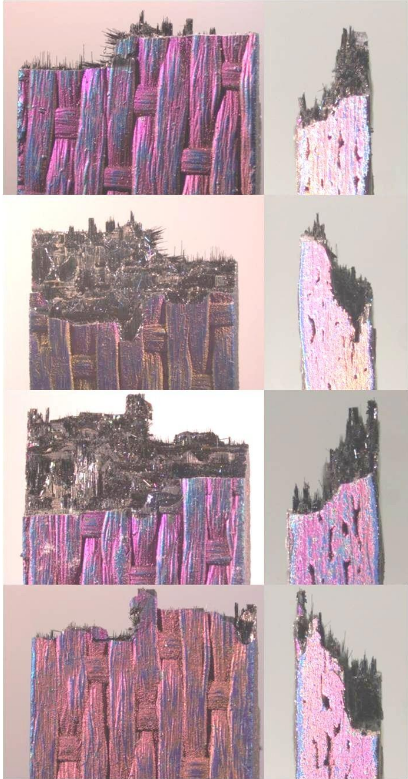
Figure 107: Optical micrographs of fracture surface of specimen P5-7 tested in fatigue at 1.0 Hz in air at 1200°C. \sigma_{\max} = 130 MPa, N_f = 70,309 , t_f = 19.5 h.
