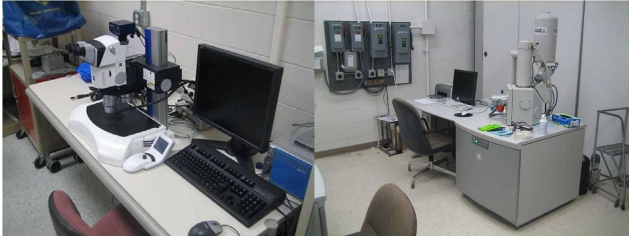
Figure 17: Zeiss Stemi SV II optical microscope (left) and Quanta 200 scanning electron microscope (right).
