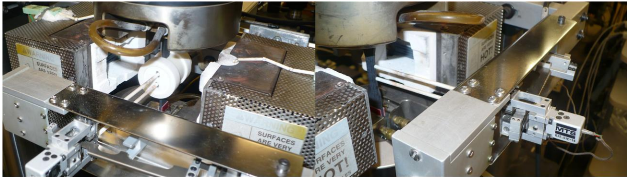
Figure 15: Test specimen mounted for steam (left) and air (right) with extensometer attached
