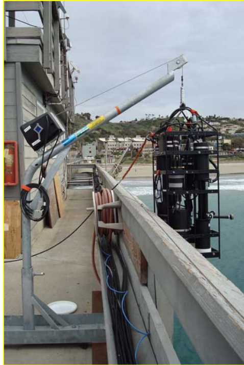
Figure 2. The OPL optics/physics profiling package (for details, see Fig. 1) being deployed from Scripps Pier during the RaDyO field testing phase in January, 2008.
