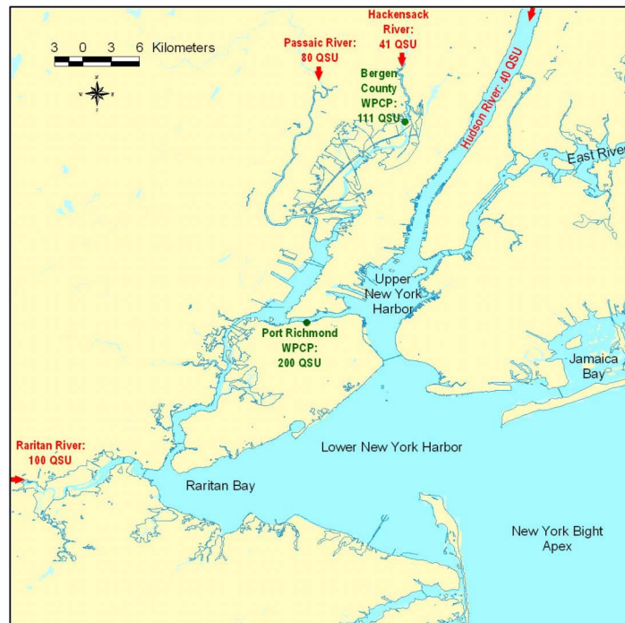
Fig. 3. Non-point source (reverine, in red) and point-source (treatment plants, in green) CDOM end-point strengths, in quantinine salinity units (QSU), as simulated in the Stevens IT NYHOPS model, based on observation-derived guidance by the Umass Boston team.
