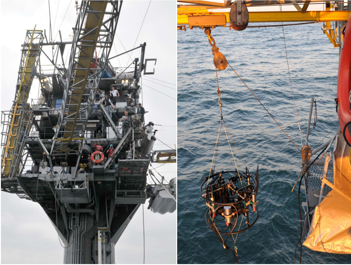
Figure 3. Deployment of the Underwater Porcupine Radiometer System from FLIP during the experiment in the Santa Barbara Channel in September 2008.
