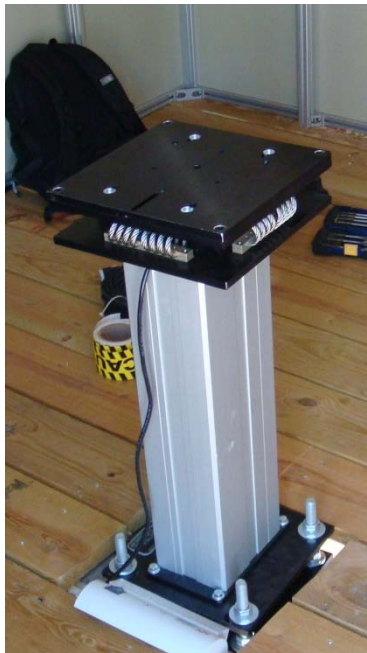
Figure 61: Pier with Vibration Isolation System
