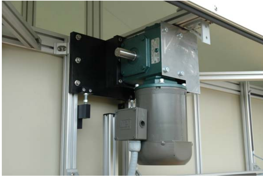
Figure 63: Roof Motor with Worm Gear ( photo credit: Pier-Tech, Inc 2007 )
