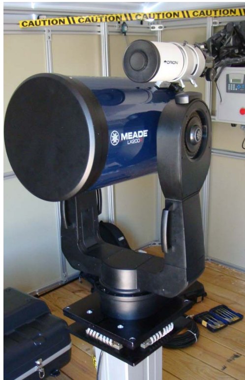
Figure 62: Telescope Mated to Pier
