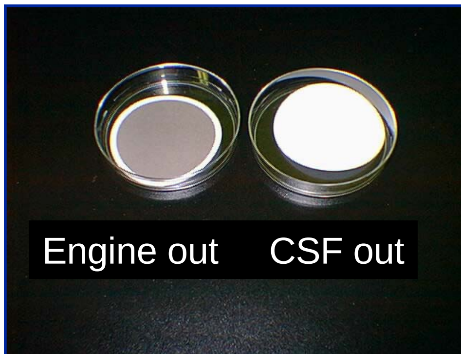
Figure 2.4 Effectiveness of a CSF in Reducing Total Particulate Mass
