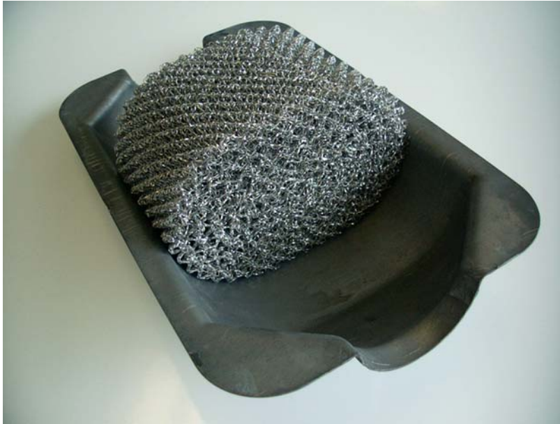
Figure 2.1 ESW Particulate Reactor Cut-away
