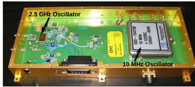
Figure 1. (a) Block diagram of the synthesis scheme for locking the 2.5-GHz STW oscillator to the 10-MHz quartz oscillator. The PM noise floor of PLL frequency synthesizer inside the loop BW is approximately -87.0 dBc/Hz when the input frequency of the phase/frequency detector = 400 kHz, and the output frequency of the oscillator = 2.5 GHz. (b) Picture of phase-locked oscillators module.
