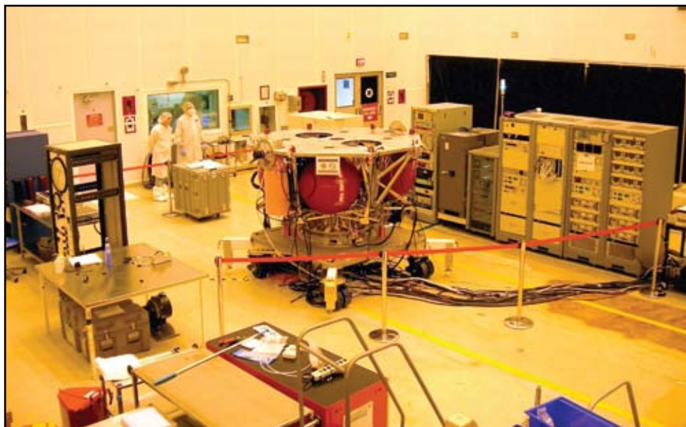
FIGURE 8(a) Electrical testing in the SMAB high bay at CCAFS.
