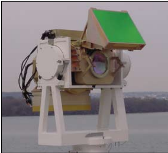
FIGURE 12 DASIRST sensor (bronze-colored assembly) mounted on pan-tilt positioning system.
