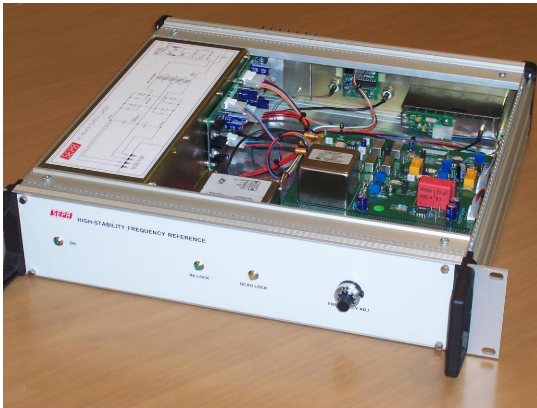
Figure 7. High-stability frequency reference, inner view showing Rb and OCXO.
