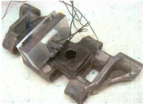
Fig. 5: Tank shoes with prototype fixture attached.
