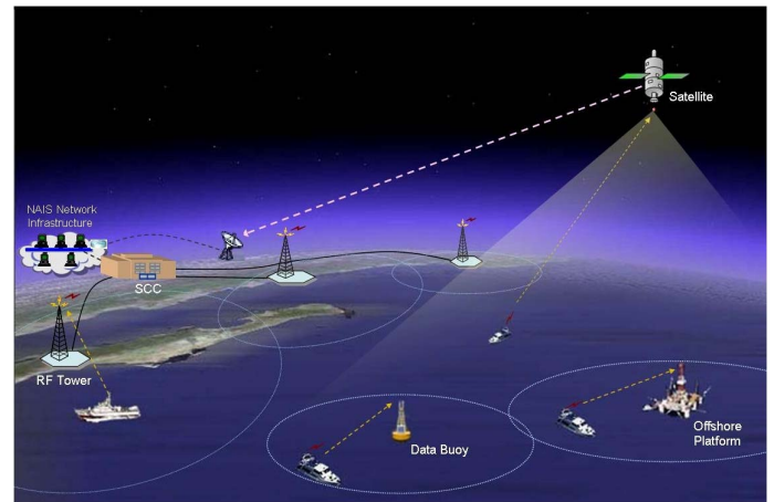
Figure 6. Schematic diagram of N-AIS Increment 3. Satellites and buoys acquire AIS position reports from regions out of view of shore based receive towers. The goal of Increment 3 is to be able to track AIS targets out to 2000 nm.
