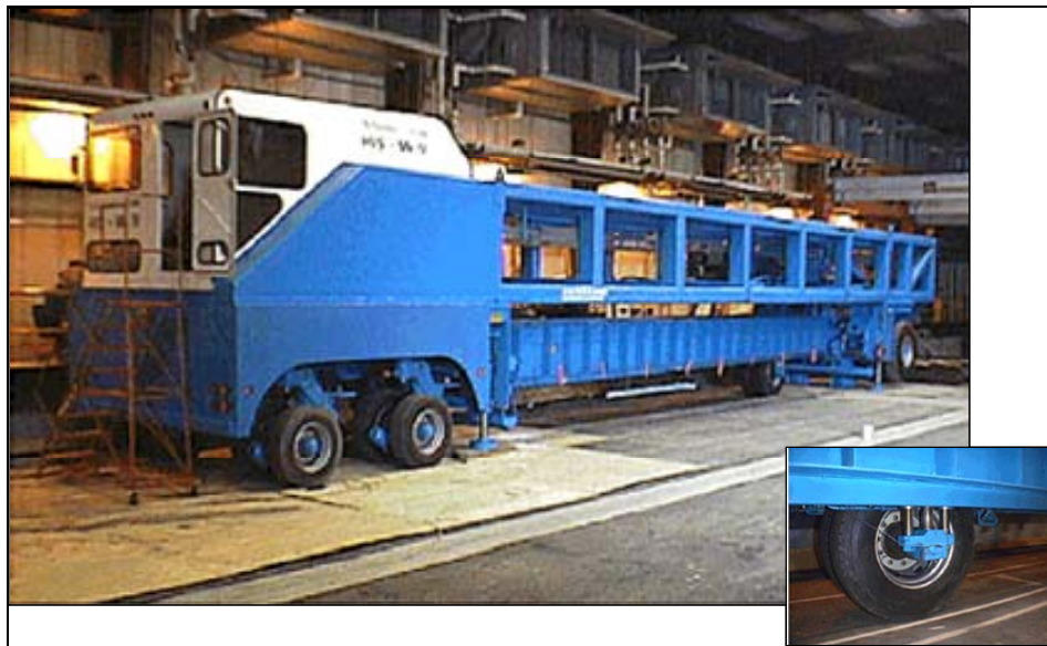
Figure 6. Mark IV heavy vehicle simulator (HVS) mounted with dual truck tires (inset).
