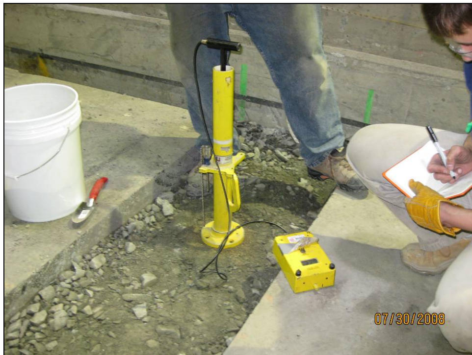
Figure B11. Clegg Hammer used to measure soil strength on test sections.
