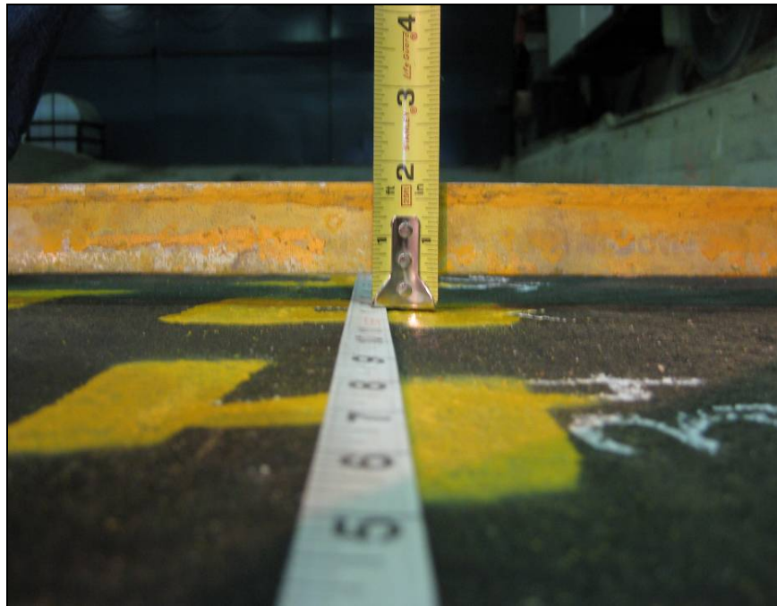
Figure B6. Rut depth near Geogrid strain gage locations in Test Section 7.
