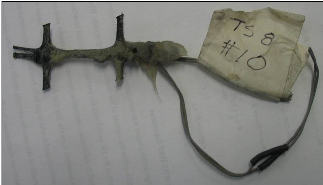
Figure B28. Close-up of Geogrid strain gages hand-cut from TS 8.
