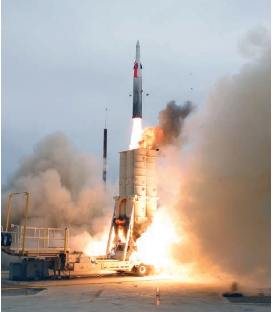
Arrow-2 antiballistic missile launches to intercept incoming target missile as part of a joint U.S.-Israel test program
