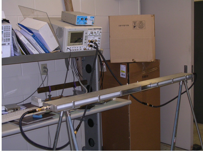
Figure 101. Equipment used for stripline measurements. The waveguide is the large stripline described in Section 3.6.3. TDR measurements are taken using an Agilent 86100B Wide-Bandwidth Oscilloscope with an Agilent 54754A Differential TDR Module.
