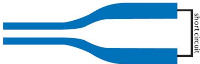
Figure 2.2: A tapered quarter wave transmission line utilizes wide width and large gap spacing when the current is high (voltage is low) and narrow width and small gap when the voltage is high (current is low).
