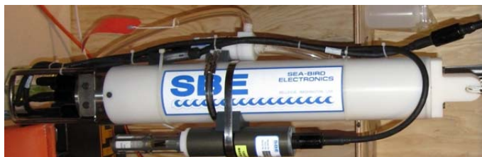
Figure 9. Sea-Bird Electronics SBE 19plus V2 with SBE18 pH sensor. As deployed at APLIS 2009.
