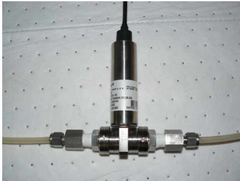
Figure 21. Differential Pressure (DP) cell
