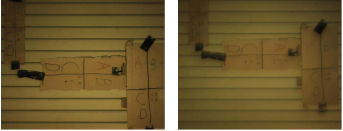
Figure 4.4: (Left) Image acquired with the fore optic, second lens ( Lens 1 ), iris diaphragm, and the ThorLabs DCC1645C ( Camera 1 ). The iris diaphragm is closed down to 8.3mm. (Right) Image acquired with the fore optic, second lens ( Lens 1 ), iris diaphragm, Mirror 1 , and the ThorLabs DCC1645C ( Camera 1 ). Some reduction in image quality is seen due to the iris diaphragm not being centered perfectly on the lens.
