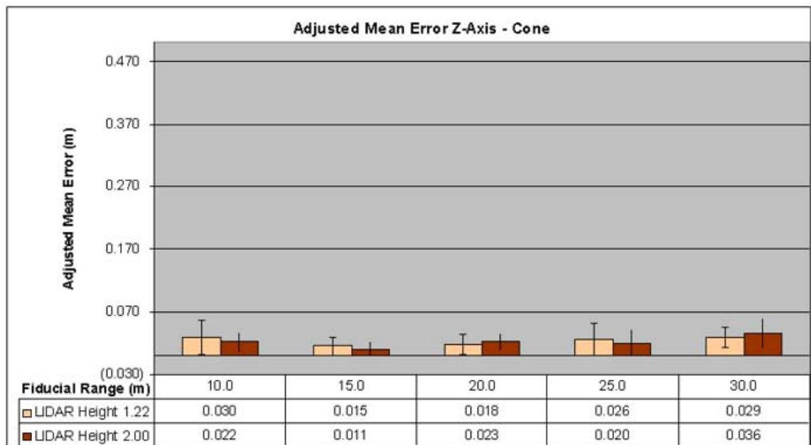
Figure 18. Adjusted mean error for Z-axis position estimate – cone.
