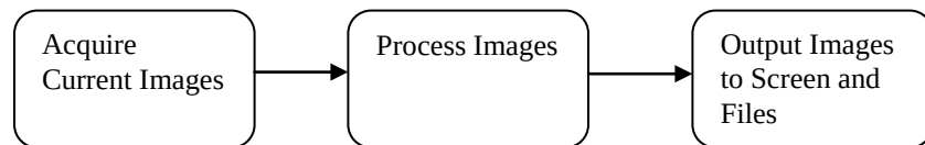
Figure 47. Example of a possible pipeline implementation to increase speed.
