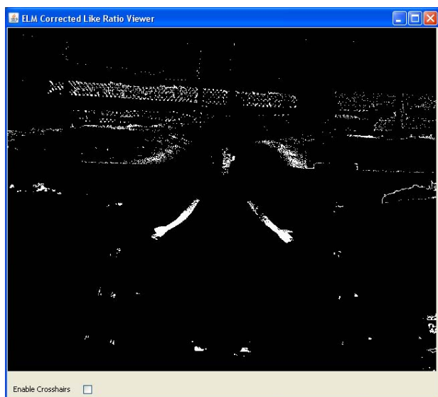
Figure 32. Output of the likelihood ratio test algorithm and ELM. Notice that snow is still declared as skin, shadowed regions of skin are not identified, and the corners of the image are also declared as skin.
